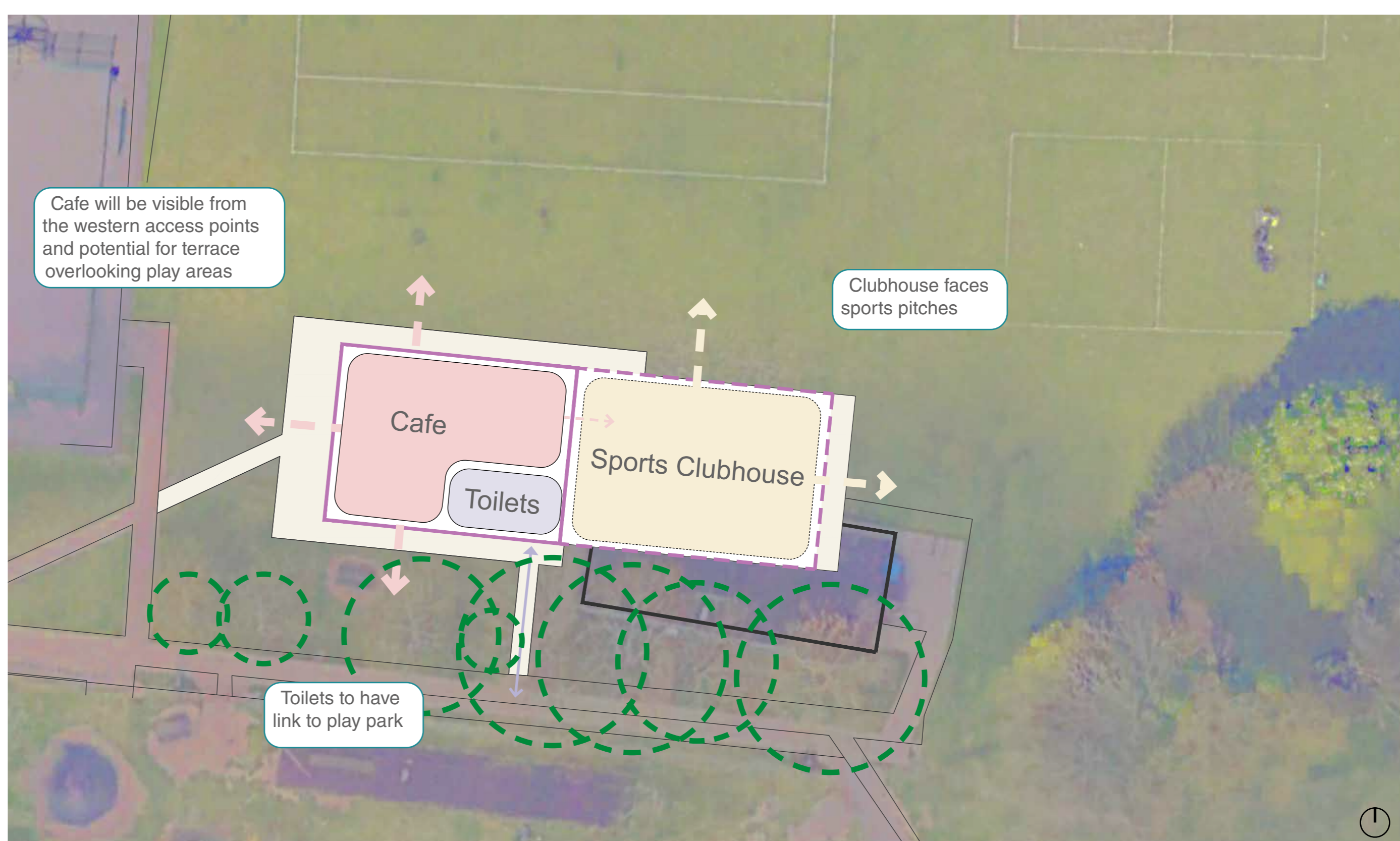
Site plan - proposed building components and their relationship to the trees (green dash circles) and existing building footprint position (black line)
