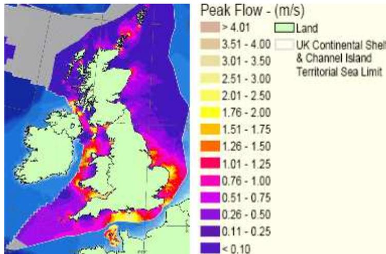
Figure 66 – Predicted mean spring peak current velocities in UK waters
