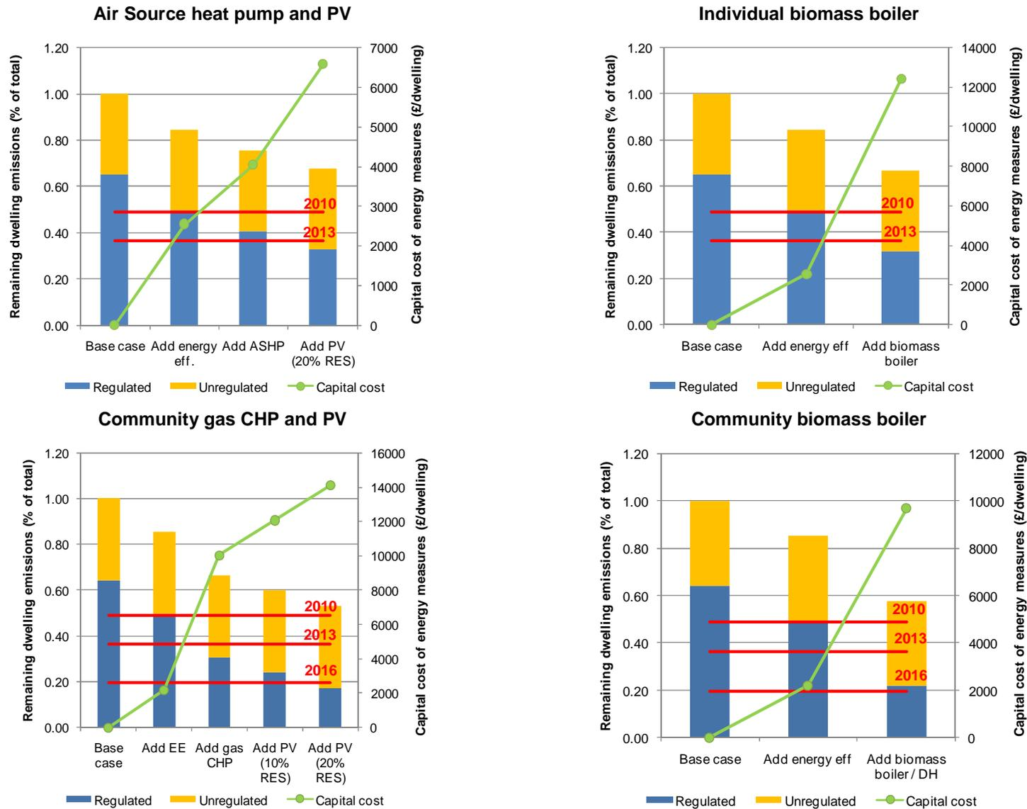
Figure 84, Progressive CO<sub>2</sub> reduction and cumulative capital cost build up as components added to energy systems (based on a 3bed semi)
