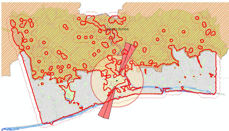
Figure 60, Map identifying restrictions on wind turbine deployment due to built environment. Solid red lines indicate a 100m separation distance from buildings (typical for a small scale turbine < 100kW). Dotted red lines indicate a 400m separation distance (typical for MW-scale turbines).
