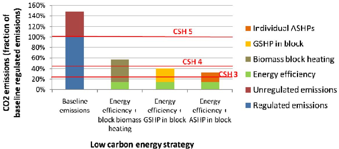
Figure 49 – CO<sub>2</sub> reductions achievable through deployment of a range of block based low carbon energy strategies
