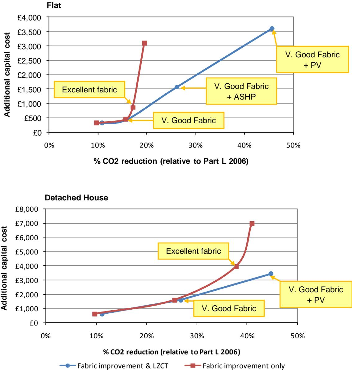
Figure 19, Comparison of cost of achieving increasing levels of CO<sub>2</sub> reduction through improvements to the dwelling fabric (i.e. U-values, air permeability etc.) alone with cost of achieving similar levels of reduction through combination of fabric improvement and low carbon technologies.
