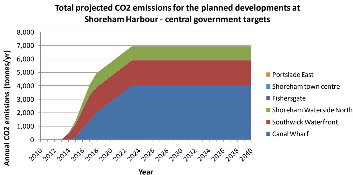
Figure 2 - annual CO<sub>2</sub> emissions which will result from the Shoreham Harbour new build developments if all buildings are built to the building regulations standard in force at the time of build.
