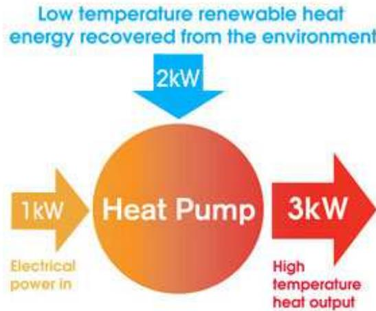
Figure 46 – heat pumps provide more heating energy than they consume in electrical energy. The ratio between heat energy out and electrical consumption is known as the coefficient of performance (COP). The heat pump illustrated above has a COP of 3
