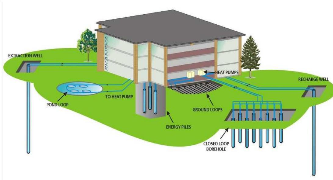
Figure 48 – schematic diagram of potential heat pump systems – high density developments at Shoreham Harbour via require boreholes to be drilled
