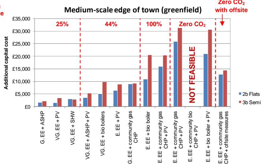
*Figure 78 – Capital cost of achieving varying CSH energy and CO<sub>2</sub> standards for a range of representative development types (Key to abbreviations: G – Good, VG – Very Good, E – Excellent, EE – Energy Efficiency package)*
