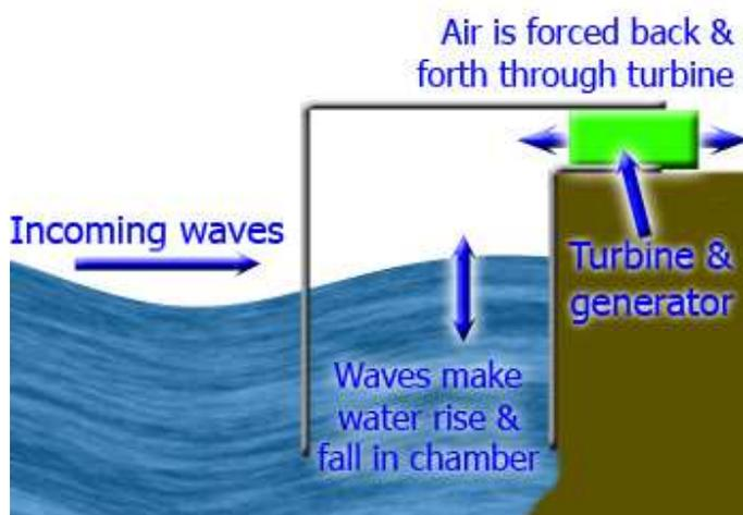
Figure 68 – Operation of a wave power generation unit
