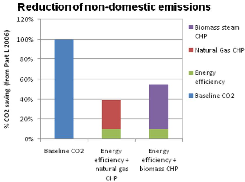
*Figure 44 – CO<sub>2</sub> reductions achievable in the non-domestic sector through deployment of biomass and natural gas fired CHP engines and district heating systems at Shoreham Harbour*
