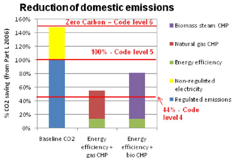
Figure 43 – CO<sub>2</sub> reductions achievable in the domestic sector through deployment of biomass and natural gas fired CHP engines and district heating systems at Shoreham Harbour
