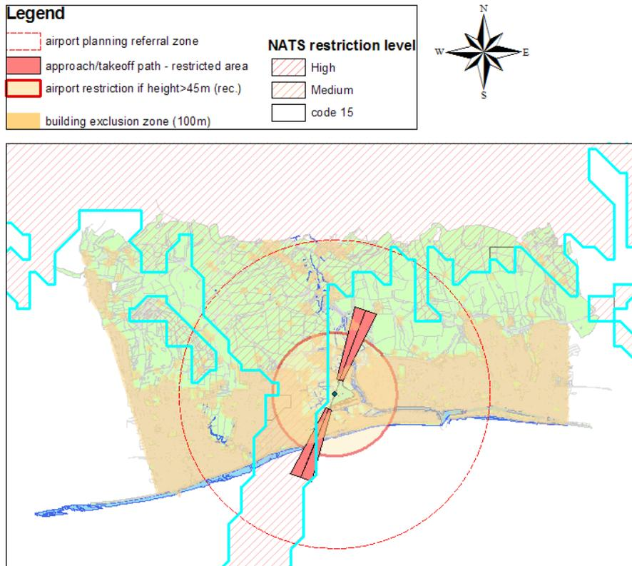
Figure 57, National Air Traffic System (NATS) restricted areas for wind turbine installations.
