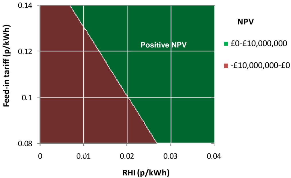
Figure 42, Plot of the ranges of level of renewable feed-in-tariff (FIT – subsidy for renewable electricity) and renewable heat incentive (RHI – subsidy for renewable heat) at which the Whole Harbour district heating system is expected to provide a positive return on investment.
