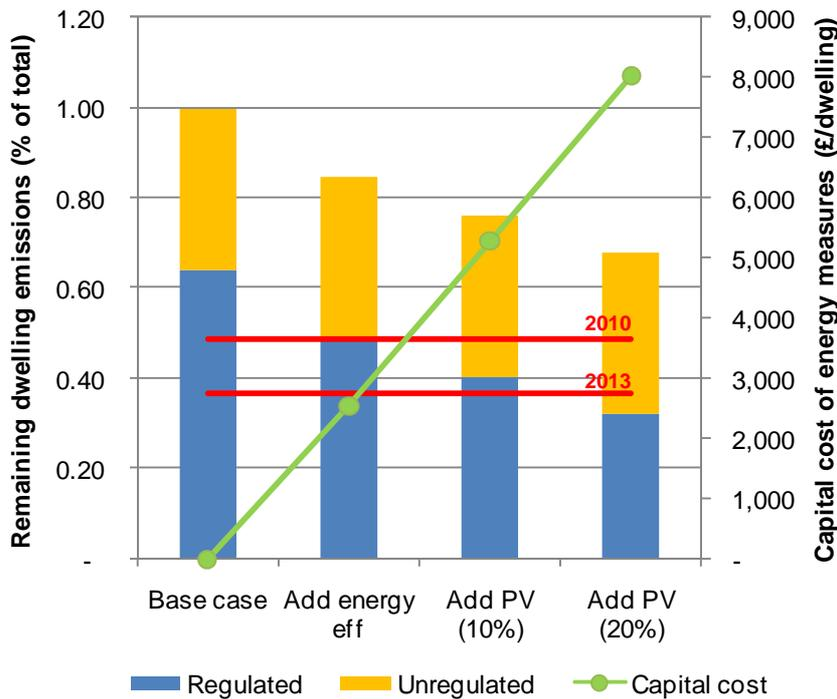
Figure 83, The progressive CO<sub>2</sub> reduction of a 3-bed semi as energy efficiency measures and then photovoltaics are added to the base case dwelling (Part L2006) is shown in the chart. The horizontal red lines indicate the CO<sub>2</sub> reduction standards expected to be introduced through the Part L in 2010 and
